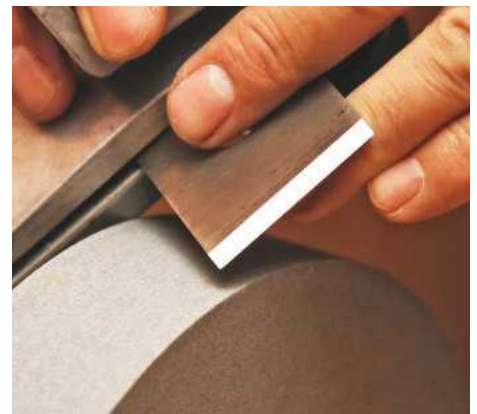
▲ The resulting grind is clean and with a very fine scratch pattern
